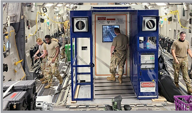
Negatively Pressurized Conex (NPC) onboard a C-17 Globemaster III
